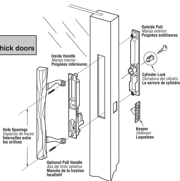
Install cylinder with key in; Twist to depress lock tab. Tab must release at edge of casting wall.
