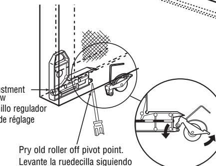
To install, keep the roller centered and use a circular arch motion to attach roller.
