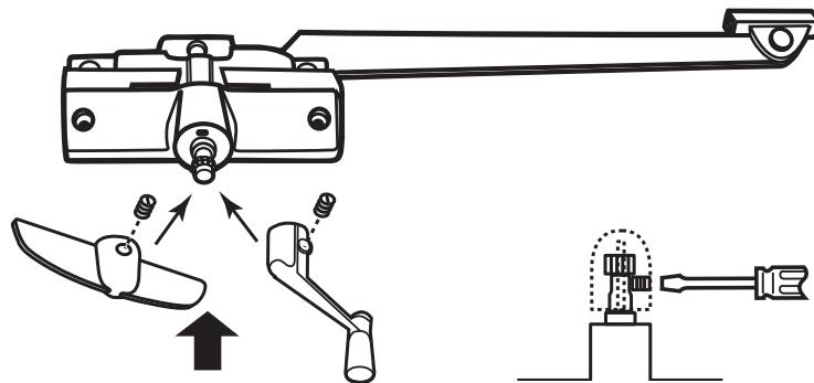
Loosen set screw on new handle and press onto stem, turning slightly until handle drops in, tighten screw.
