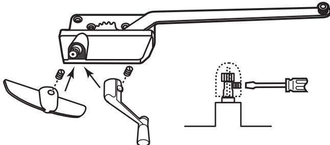
Loosen set screw on new handle and press onto stem, turning slightly until handle drops in, tighten screw.
