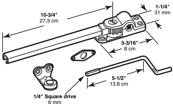
**NOTE:** Installation drawings are typical for this style of replacement part.
