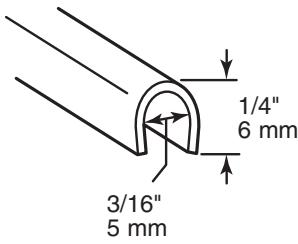
Remove the old cover and clean the track. Apply a thin bead of RTV-108 silicone adhesive. Place the track cap into position and put a 14" to 16" block of wood at least 1" thick on top, begin tapping the wood with a hammer to force the track into position. Keep moving down about 1" every couple of hits.
