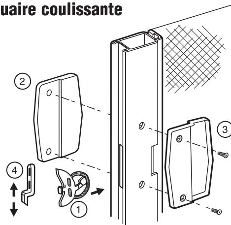
Remove old handles. Insert hook assembly (1) into latch opening and hold in position while installing outside handle (2). Be sure lever fits into latch slot in handle. Align inner handle (3) and install screws. Check for smooth operation and adjust strike (4) if necessary.
