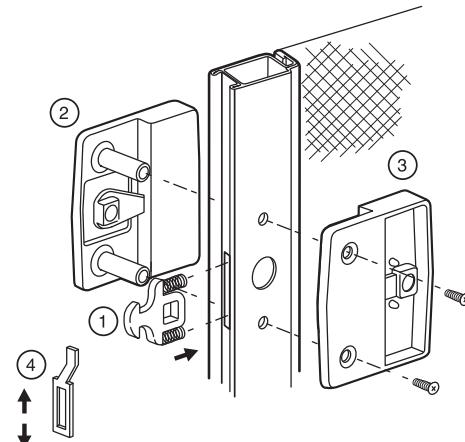
Remove old handles. Insert hook assembly (1) into latch opening and hold in position while installing outside handle (2). Be sure lever fits into latch hook. Align inner handle (3) and install screws. Check for smooth operation and adjust strike (4) if necessary.
